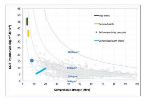
**Figure 19.** CO2 intensity index of mud bricks (B), compressed earth blocks (CEB), and rammed earth (RE) stabilised with 5–10% OPC, in comparison with data for PC concretes. Also included is the index of self-compacted clay concrete (SCCC) stabilised by 5% CSA cement. Note that the carbon footprint of the superplasticiser (~40% of that of cement) has not been taken into account (adapted from Fig. 5 of (Damineli et al. (2010))).
