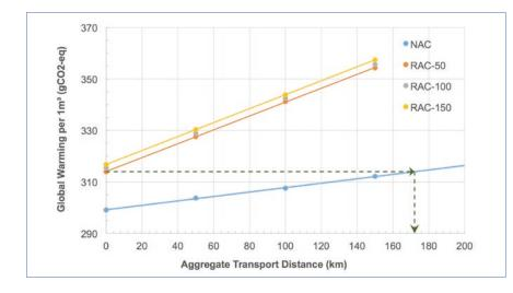
Figure 18. The effect of transportation distance on associated CO2 emissions of concretes produced with recycled aggregates and natural aggregates. The substantial difference results from tested recycled aggregates requiring much higher cement content to reach the necessary design strength [47].
