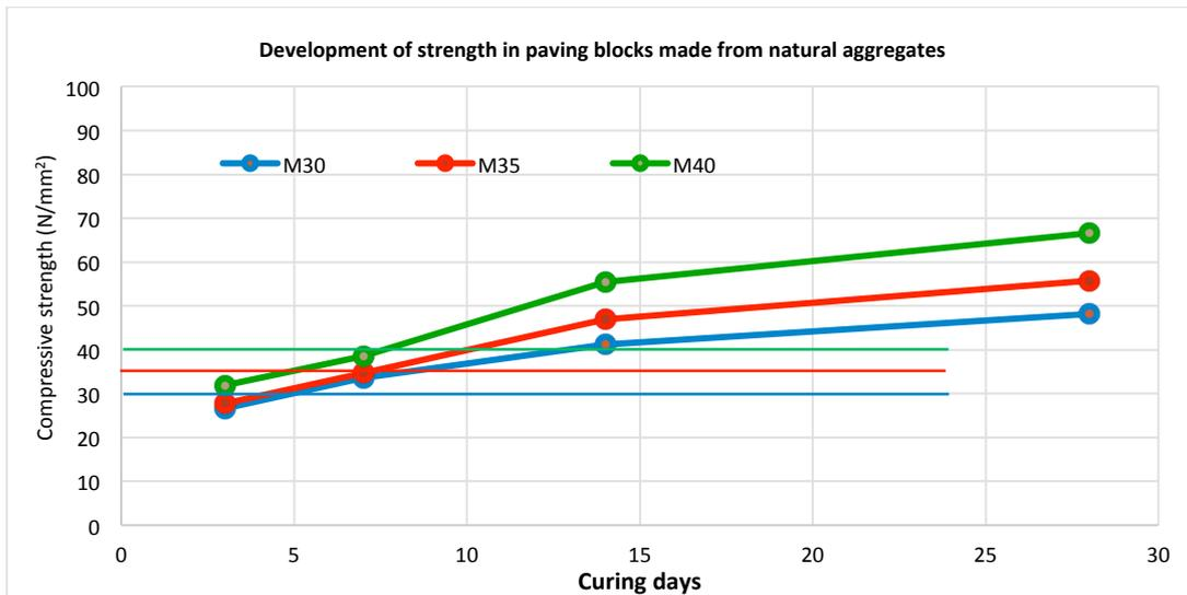
It was observed that 100% strength was achieved within 7 days. The rate of strength increase was similar in all grades of paving block. However, an average of 60% higher strength was seen in all grades for natural aggregate based paving block.
