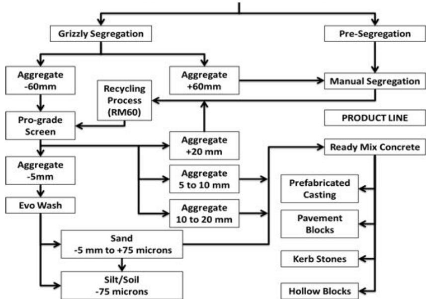
Paharganj and City. 27 collection points were identified for waste collection. Later, this was increased to 48. The facility recovers about 97% of the materials from waste for processing. Treated sewage water is used for wet processing. The C&D waste is thereafter recycled into aggregates at the waste management facility, which is in turn converted to Ready Mix Concrete (RMC), pavement blocks, kerbstones and concrete bricks. 1,200-1,400 bricks can be produced daily in an 8 hour shift.
