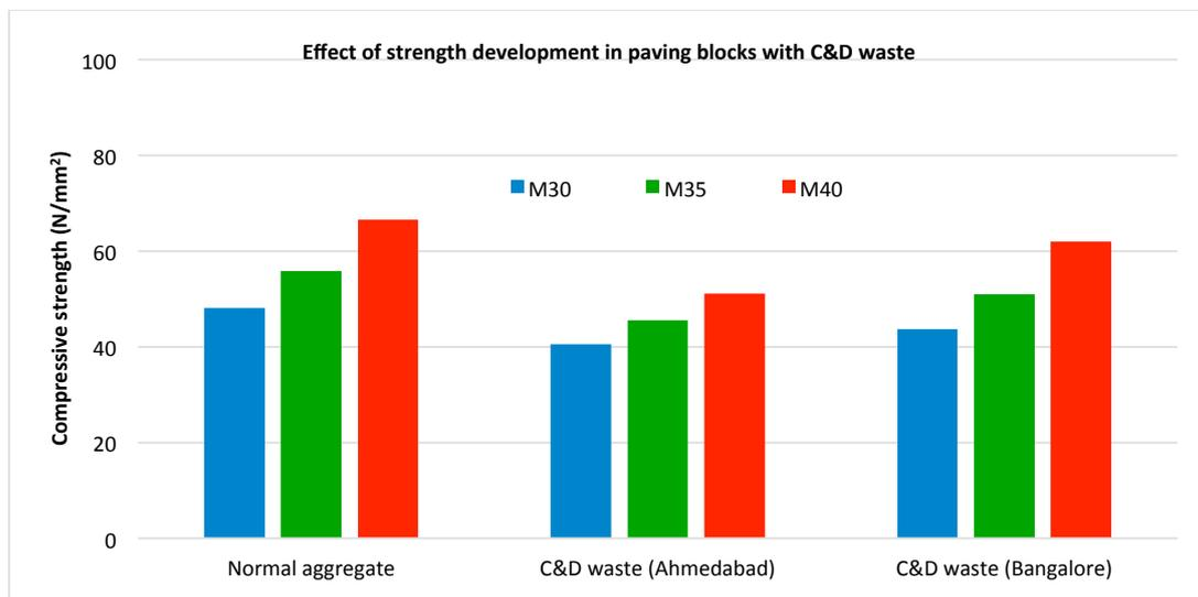
Paving block made with C&D waste from Ahmedabad and Bengaluru fulfil the properties (compressive strength) as per BIS 15658:2006. Thus, paving blocks for non-traffic, light-traffic and even medium-traffic areas can be produced with C&D waste.
