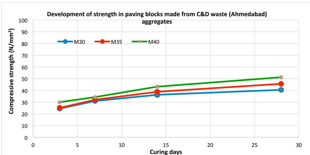
M30 grade paving block achieved 100% strength within 7 days while in M35 and M40 grade strength was achieved within 14 days. The rate of strength increase is similar in M30 and M35 grades of paving block but M40 grade paving block has an improved strength development. On an
