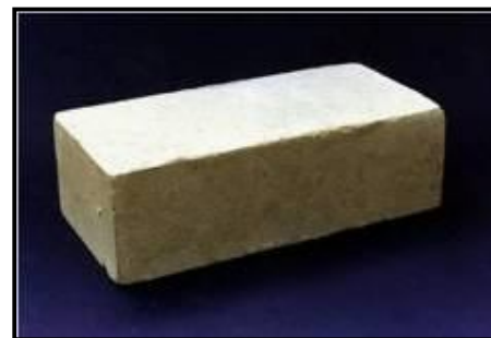
Figure 10: Sand lime Bricks
