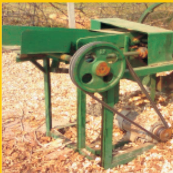
Activities like biomass cutting and chopping is done by biomass cutter
