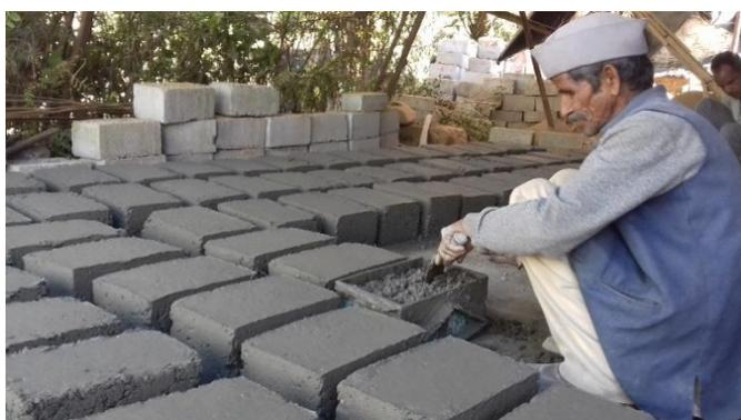
Concrete blocks are large sized masonry units made by compacting a well graded concrete mix. Since they can be produced easily using simple moulds, they are already being produced by house-builders in the mountain region. Although it is an appropriate material for localized production, there is no awareness of its basic requirements for quality- namely the correct mix and adequate
