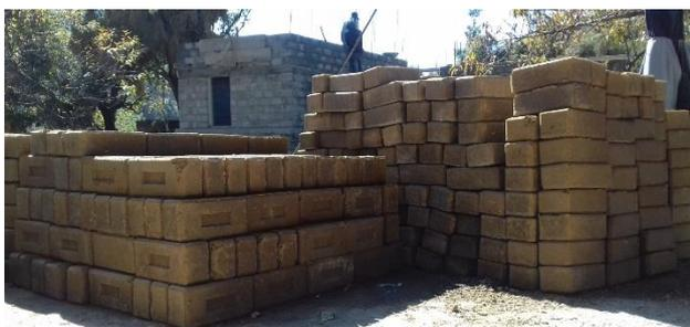
SCEB is a replacement for burnt clay bricks which are transported from more than 200 km away to rural areas. The main raw materials for SCEB – soil and coarse sand are locally available – hence SCEB are a good option for local production of masonry material. SCEB are made by compressing earth/ soil mix by simple mechanical means. The basic concept underlying compressed earth blocks is densification of the soil mix using external energy- this
