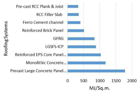
Figure 14: Embodied energy of selected roofing systems
