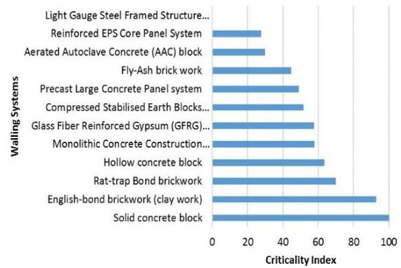
Figure 15: Critical resource use in selected walling systems
