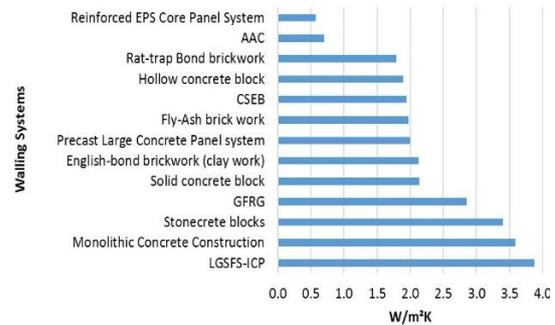
**Figure 19:** Thermal performance of selected walling systems
