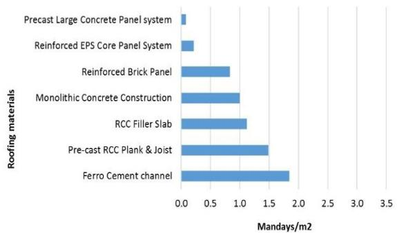
Figure 24: Job creating potential of selected roofing systems
