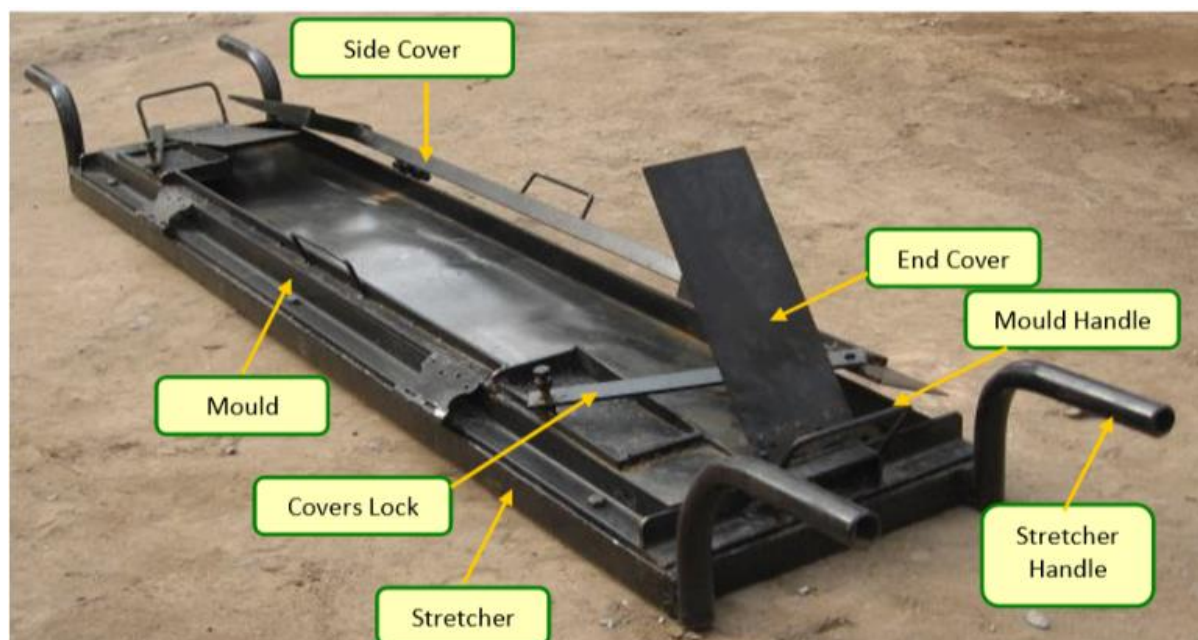
Mould used to cast planks along with the details of its various parts
