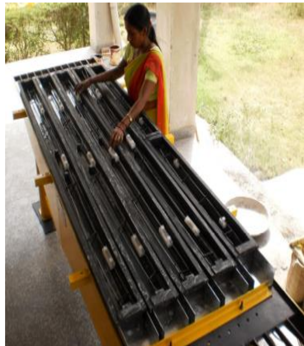
Vibrating table with five moulds and total capacity of two set of door frames in one cycle
