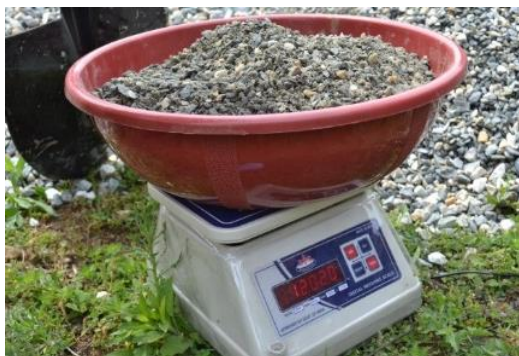
Weighing process of raw materials for the preparation of concrete mix.
