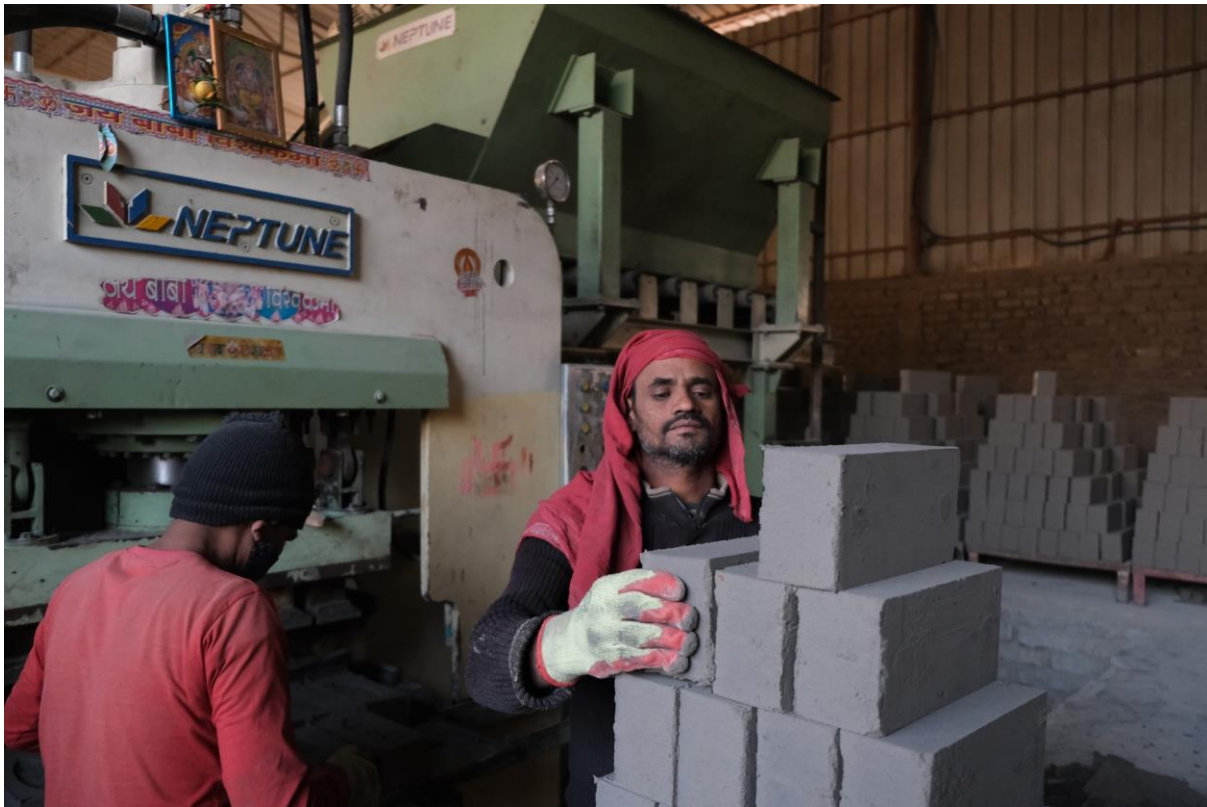
Fly Ash Brick making in progress
